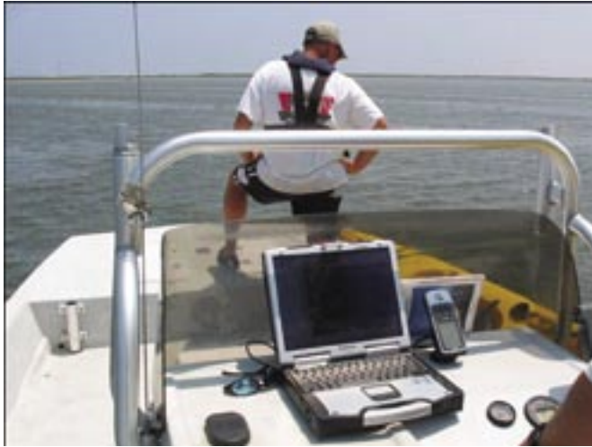
Figure 3. The field data entry set up in one of the Texas Parks and Wildlife boats. Notice the link to the GPS device, which allowed field personnel to use the digital camera imagery to navigate directly to chosen sample segments as displayed on the computer screen.
