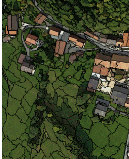
Fig. 2: Multiresolution segmentation of airborne image data: trees and meadows are of similar spectral value. They are separated because of the high difference in spectral homogeneity. Following criterion (9), the merge of a homogeneous image object to a heterogeneous image object would result in a big change of heterogeneity for the homogeneous object.
