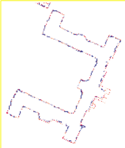
Fig. 4: Overlay of segmented building (Stuttgart Castle, subset: 200 x 250 m 2 ; blue) onto cadastral data (red) showing the satisfying geometrical accuracy of the approach
