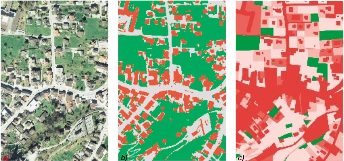
**Fig. 3** Digital orthophoto (a), classification resulting from an object-oriented multi-scale segmentation approach (b), percentage of sealed surface per parcel using the results from (b) and the existing cadastre (from Pilz 2001 with kind permission).
