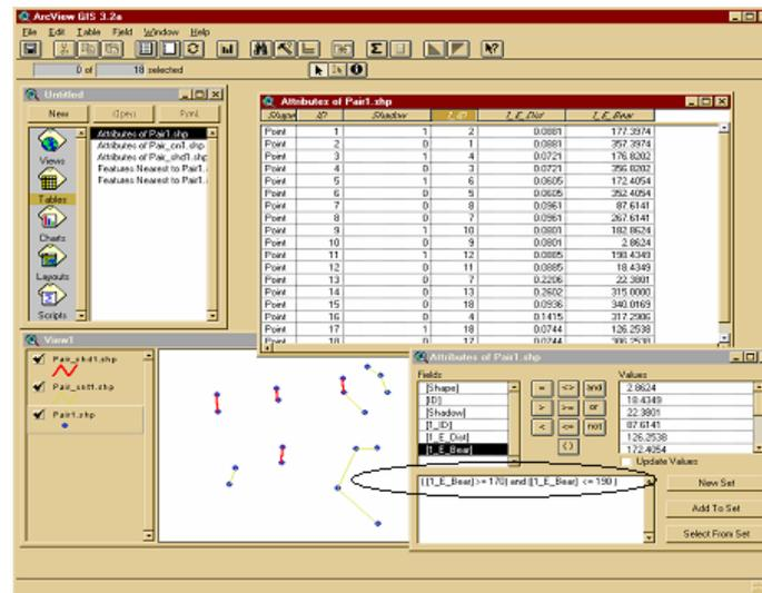
Figure 3. Finding a pair of tree shadow and the tree based on their distance and direction
