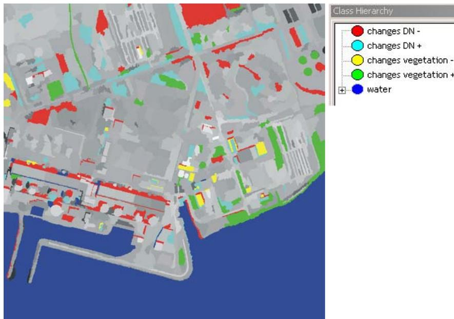
Fig. 4: Classification result for the object-oriented change detection using MAD components
