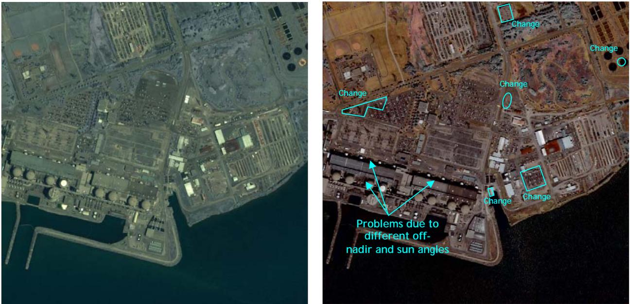
**Fig. 1:** IKONOS-2 images over Pickering Nuclear Power Generating Station, Canada, July 2000 (left) and July 2001 (right). On the left image, major changes and problems due to different off-nadir and sun angles are indicated
