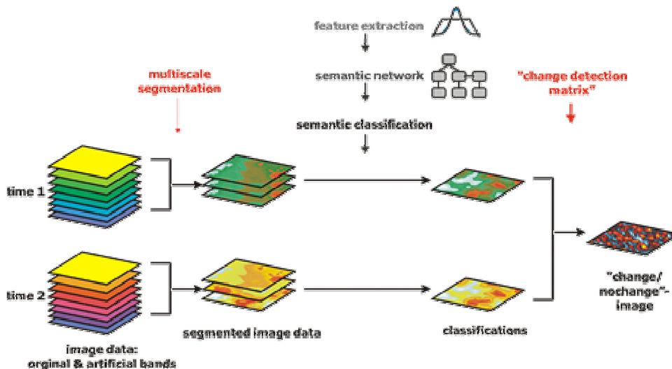
Fig. 4: Object-oriented change detection using a change detection matrix
