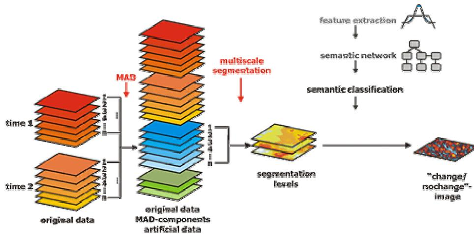
Fig. 3: Object-oriented change detection using MAD components
