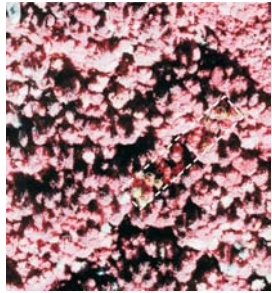
Figure 1. CIR digital orthophoto 1:10000 (~20cm GIFOV) over NPBW site 22. The markers show dominant field measured crowns: spruce (yellow) and deciduous (mostly beech, in red) with diameter of marker varying with tree height. Only crowns >15m shown. Note the variety of crown shapes, from disks to occluded crown fragments in the shape of crescents. Occlusion occurs due to mutual shadowing effects.
