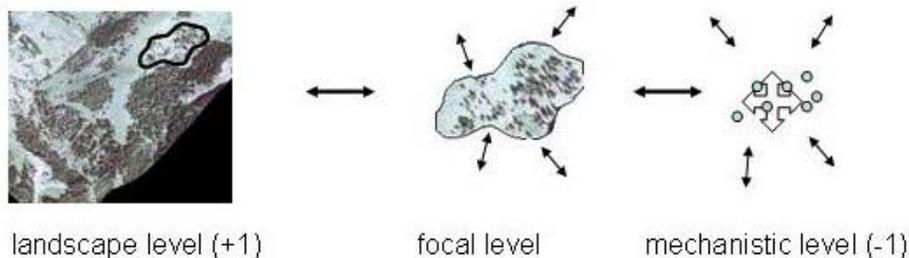
**Fig. 1:** Basic principle of multiscale, oo image analysis: Information is gained and explicitly expressed through objects, their respective super-objects (here only one level above the ‘focal level’ is shown) their respective sub-objects (here single trees) and specific characteristics of the subobjects such as their spatial arrangement, distribution, shape, size, spectral characteristics and many derived products from shape/area/distance relationships.
