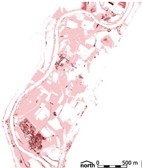
Fig. 6. Estimated financial damage map based on the IKONOS-2 land cover map. Graduated color map; dark red: high damage rates, light red: low damage rates; white: no damage or no information.
