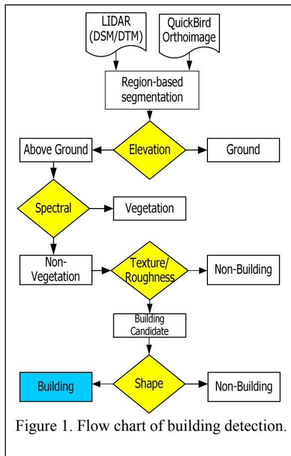
Figure 1. Flow chart of building detection.
