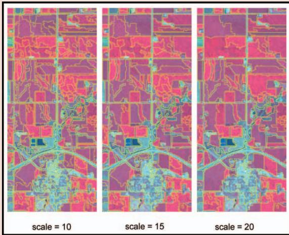
Figure 2. Segment boundaries created from the Landsat 5 image. A comparison of segment boundaries using three different scales is shown. A smaller scale (e.g., 10) creates smaller segment areas.
