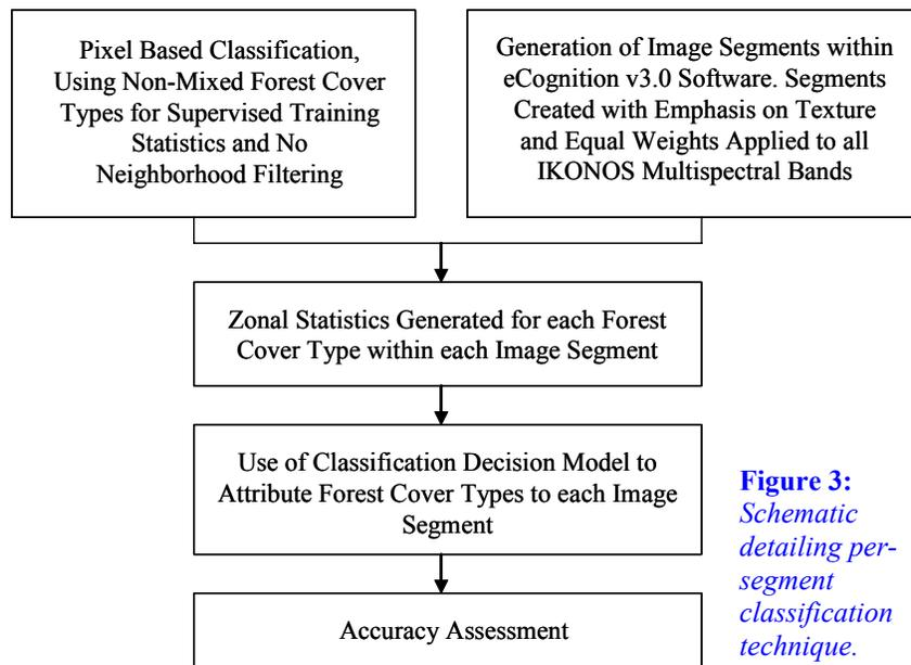
**Figure 3:** Schematic detailing per-segment classification technique.
