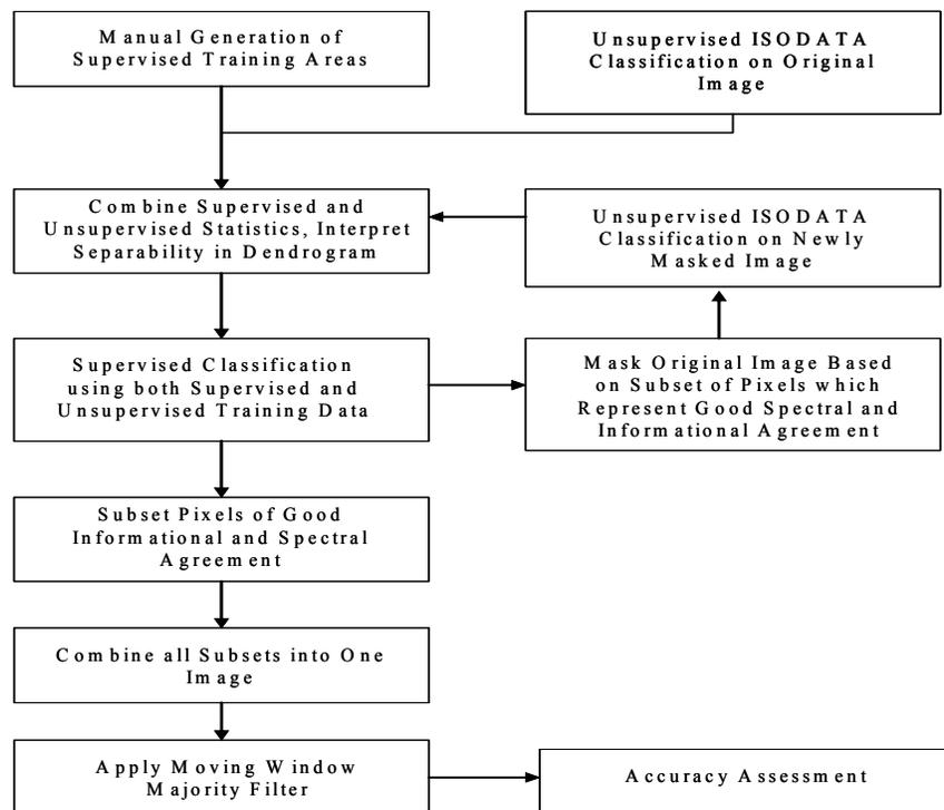
**Figure 2:** Schematic detailing per-pixel classification technique.
