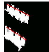
Figure 2. Detection of roof dominant lines with Progressive Probabilistic Hough Transform (PPHT): white area represents building roofs classified from Quickbird imagery; red line shows detected roof dominant lines
