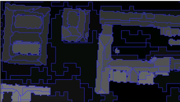
Figure 8: Segmentation (IPF and eCognition, scale parameter 30, channels 5, 120)
