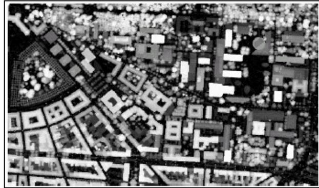
Figure 1: nDSM from laser data (first pulse mode)
