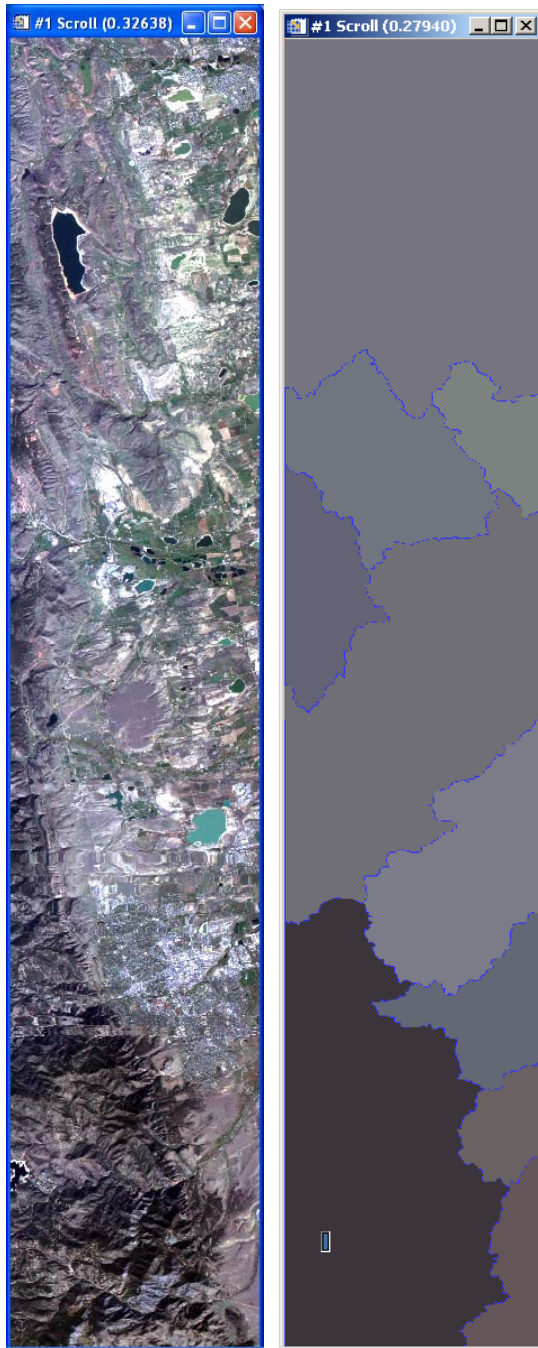
Figure 5: Left: True Color AVIRIS Image. Right: eCognition 10-segment image. Figures 6 and 7 and Table 2 show further segment analysis details.
