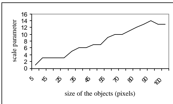
Figure 2: variation of the scale factor as a function of the size of the objects in the image.
