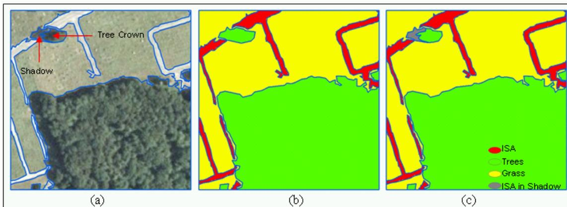
**Figure 3.** a) an example of spectral similarity of tree crowns and the shadow in a true color orthophoto; b) the result of image segmentation without considering the shadow effect, in which shadow covered ISA could not be separated from tree crowns that caused the shadows; c) the result of segmentation using the shadow-effect submodel.
