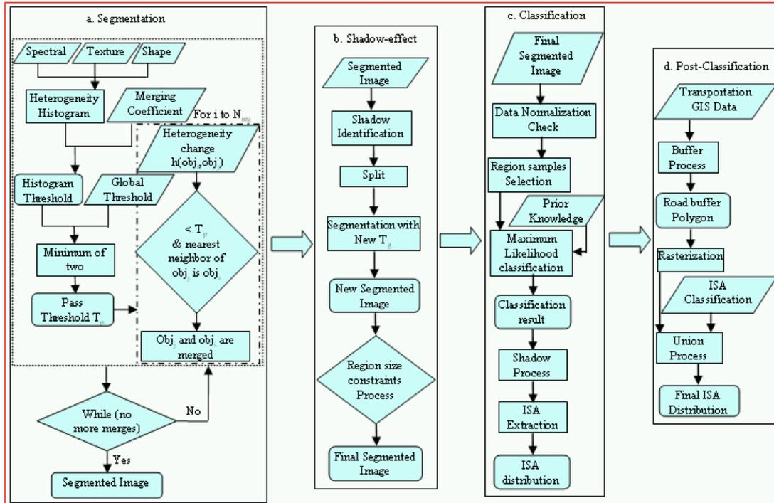
**Figure 2.** The flowchart of ISA extraction modeling. a) segmentation submodel; b) shadow-effect submodel; c) classification submodel based on segmented image; and d) post classification.
